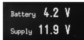
The instrument will only start if the battery voltage is greater than 3.6 Volts and the supply greater than 7 Volts. You must connect the +12 Volt power supply from the Power Portal or similar and wait until the battery is sufficiently charged. The red light will appear when external 12 Volt power is connected and the battery is charging.
