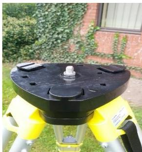
1. The Microphone Boom screws onto the threaded stud in top plate of the Tripod
