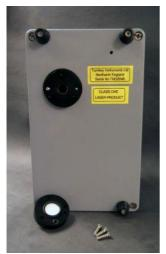
Turnkey's monitors require a flow and filter check every 3 months (later models have an inbuilt flow stabiliser, consult technical support if unsure). This is a simple procedure, which can be easily carried out following the Turnkey filter change flow chart.
