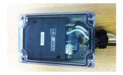
Remote GSM modem - Dust monitor end.
